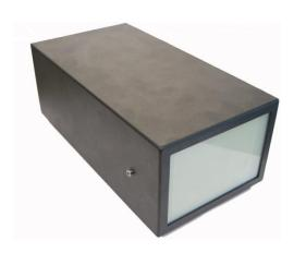
LTX-310B is a self-contained microwave transmitter for use with the LRX-310B receiver. The output is pulse modulated to identify one of 36 channels arranged in six groups of six. The group is set at the factory and you can select one of the six channels in that group from an external rotary switch.
